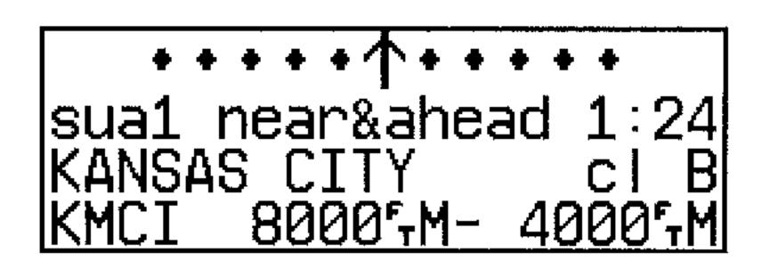
The GPS 155XL's key also provides access to Special Use Airspace information that you are currently being alerted to.
